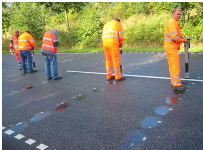
Figur 3. Foto from measurements with Sobo20. Every one do 8 measurements across the road.
